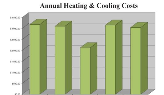
What caused the dramatically reduced energy use? Buildings 1,2, 4, and 5 are insulated with fiberglass. Building 3 is insulated with cellulose *to the same R-value*.
